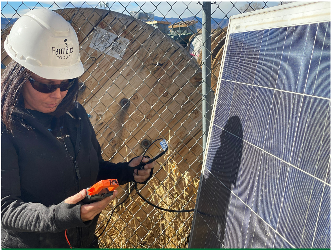
Adrienne Cloud tests the solar panel voltage output with a multimeter.
