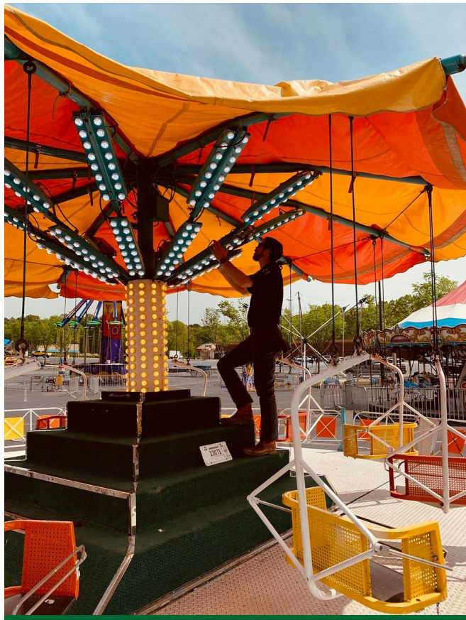
Daniel Brown inspecting a carnival ride for proper setup, missing and damaged components and current licenses as part of the public safety program.
